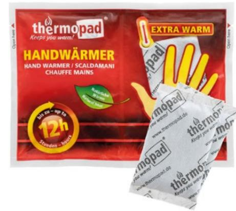
The THERMOPAD warmers work with a substance which reacts with air oxygen. As soon as you remove the warmer from its cover, the substance starts to react with oxygen and produces heat for 5 – 12 hours, depending on the type of warmer and outer conditions.
